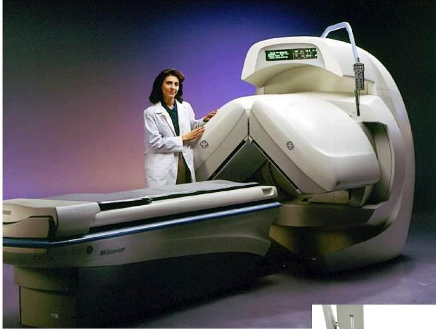
**Gamma camera** in a mammographic configuration to provide high-resolution, functional images
